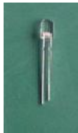
Gambar 7. Infrared Led (Sumber: Everlight, 2016: 1)
