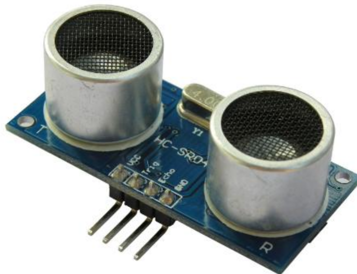
Gambar 9. Modul ultrasonik HC-SR04 (sumber: Cytron Technologies, 2013: 1)
