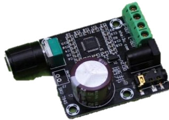
Gambar 12. Modul Amplifier PAM8610
