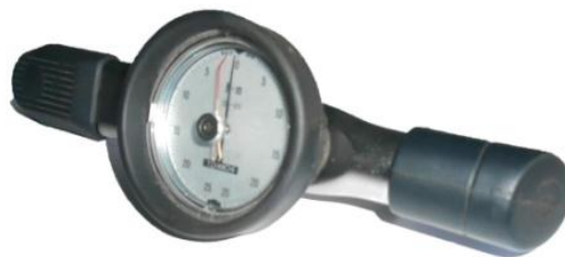
Gambar 8. Torque Wrench model dial indikator
