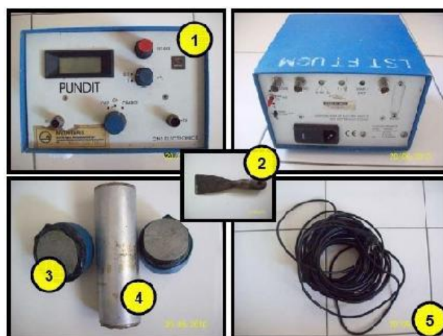
Gambar 40. Ultrasonic Pulse Velocity (UPV) (Sumber: Faqih, 2014)
