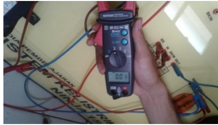
Gambar 61. Mengukur DC battery charging ampere
