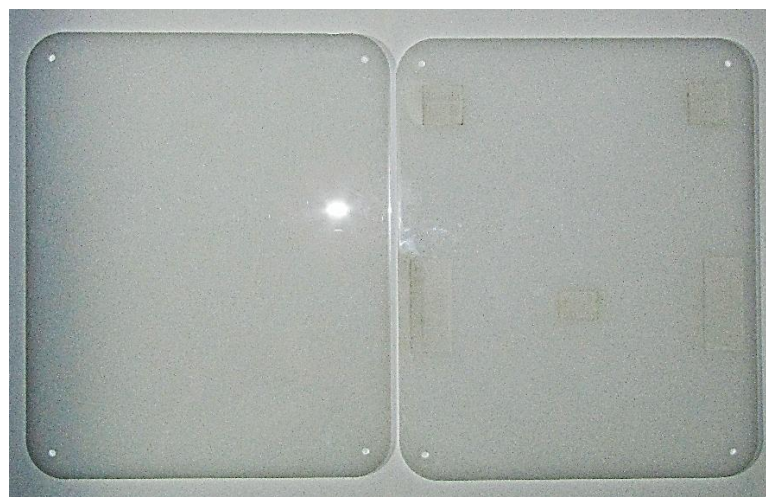
Gambar 30. Hasil Cutting Laser Acrylic Putih
