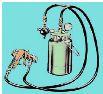
Gambar 11. Spray Gun Tipe Pressure-Feed (Gunadi, 2008)
