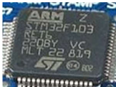
Gambar 12. Mikrokontroler ARM Cortex STM32F103RE (sumber: Futurlec, 2015)
