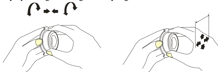
Gambar 6. Pengujian release bearing
