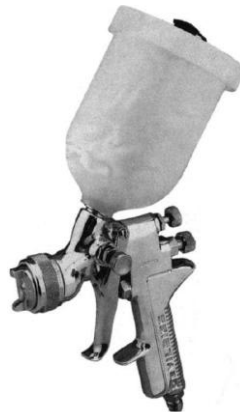
Gambar 36. Gravity Feeg Spray Gun (Robinson, 2005:584)
