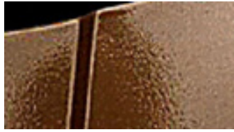
Gambar 33. Cacat kulit jeruk ( http://pc.dupont.com/dpc/en/US/html/visitor/s/trouble/PDSG_OrangePeel.html )
