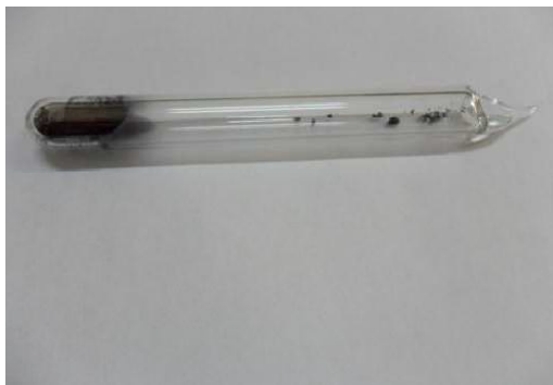
Kapsul Kristal \text{Pb}(\text{Se}_{0,6}\text{Te}_{0,4})
