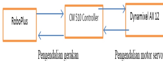
Gambar 4. Diagram blok sistem robot bipedal
