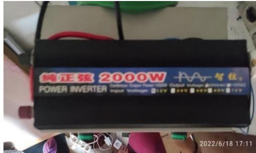
**Gambar 19.** Inverter PSW 2000 Watt
