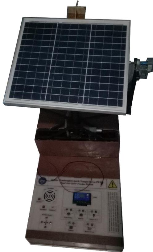
Gambar 4. Trainer PLTS dual axis solar tracking system
