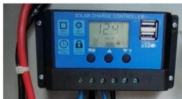
**Gambar 3.** Solar Charger Controller (SCC)
