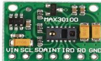
Gambar 5. Sensor BPM ( max30100 pulse oximeter heart-rate sensor module ) (Sumber: Dokumentasi Pribadi)
