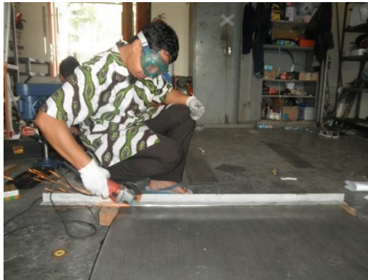
Gambar 1. Pemotongan Plat Perforated Stainless Steel (Fe+Cr)
