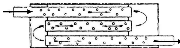
Gambar 42. Three Pass Tube Type Muffler Sumber: Ver & Beranek (2006: 35)
