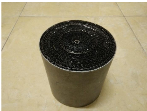
Gambar 12. Metallic Catalytic Converter Plat Tembaga Berlapis Krom
