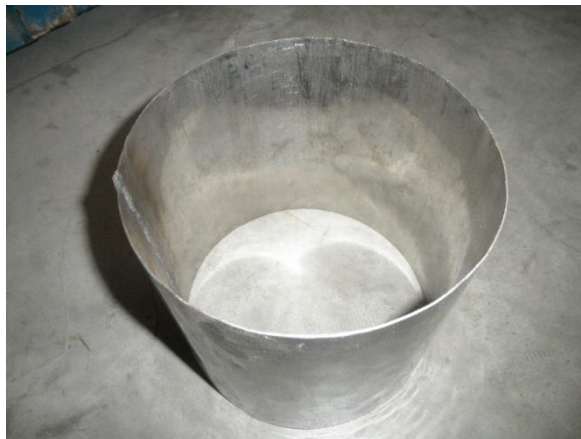
Gambar 5. Tabung Diesel Particulate Filter (DPF)
