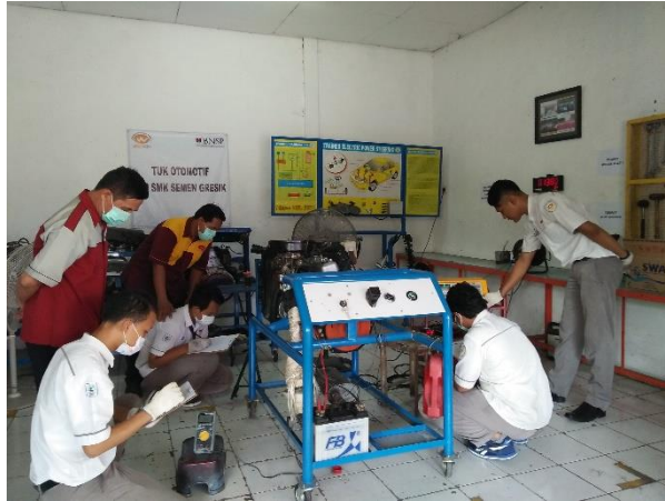
Gambar 4. Pengujian Metallic Catalytic Converter Tembaga Berlapis Krom di SMK Semen Gresik
