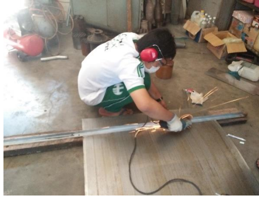
Gambar 1. Pemotongan Plat Perforated Stainless Steel (Fe+Cr)
