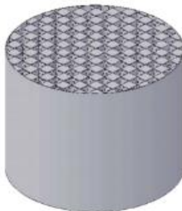
Gambar 62. Diesel Particulate Filter Berbahan Dasar Plat Stainless Steel
