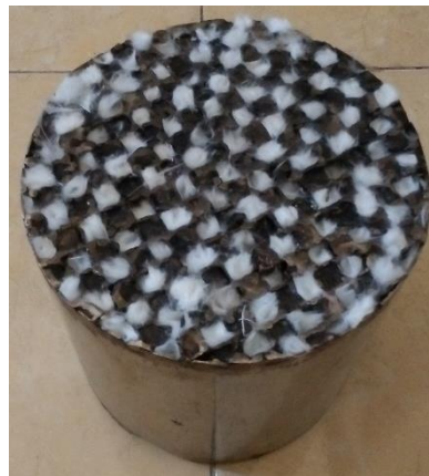
Gambar 106. Diesel Particulate Filter (DPF) Berbahan Dasar Plat Stainless Steel dan 150 gr Glasswool
