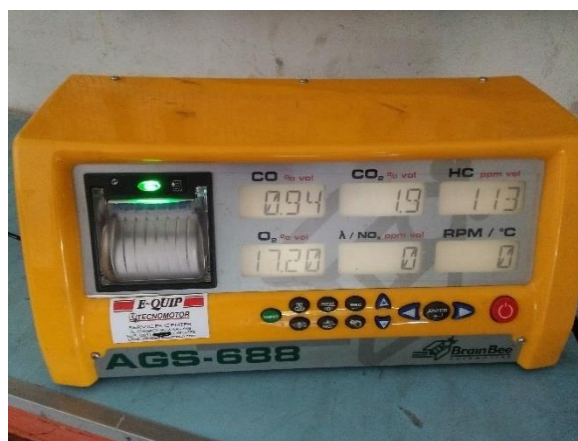
Gambar 2. Hasil Uji Emisi di Exhaust Gas Analyzer
