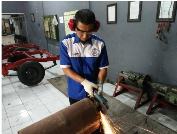
Gambar 1. Pembuatan Three Pass Tube Type Muffler
