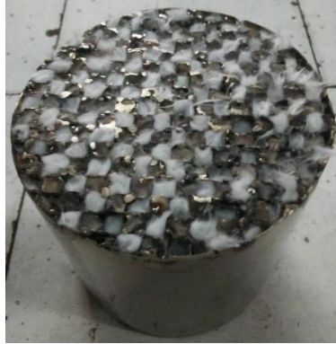
Gambar 68. DPF Berbahan Dasar Plat Stainless Steel dan 110 gr Glasswool
