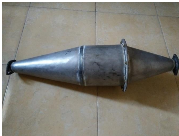
Gambar 9. Diesel Particulate Filter (DPF) Casing
