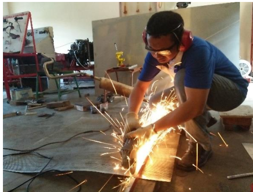
Gambar 1. Pemotongan Plat Perforated Stainless Steel (Fe+Cr)
