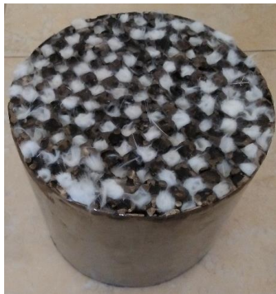
Gambar 132. Diesel Particulate Filter (DPF) Berbahan Dasar Plat Stainless Steel dan 130 gr Glasswool
