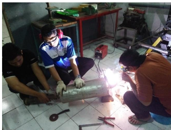
Gambar 2. Pengelasan Elbow Muffler
