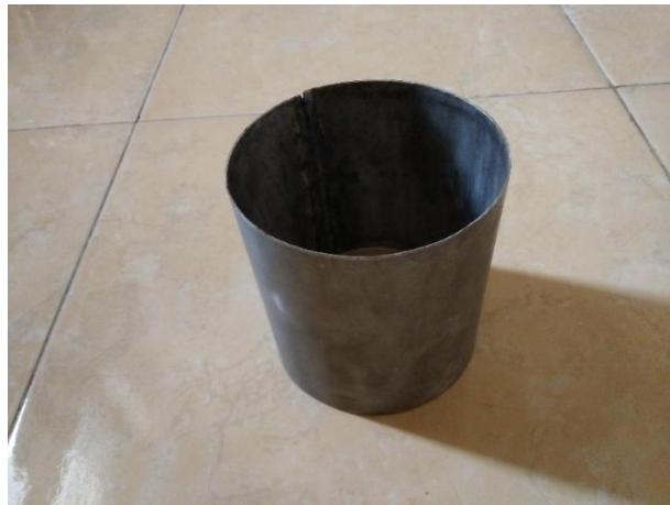
Gambar 11. Tabung Metallic Catalytic Converter
