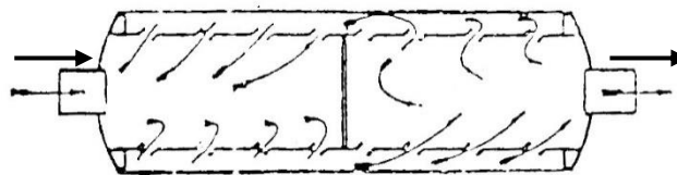
Gambar 41. Louvre-type Muffler Sumber: Ver & Beranek (2006: 35)
