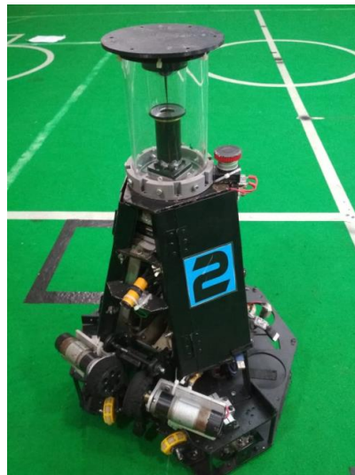
Gambar 24. Hasil Pembuatan Robot Three Omni-Directional Wheels
