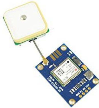
Gambar 8. Receiver GPS (Sumber: Andi Sunyoto, 2013: 1)
