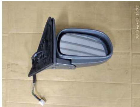
Gambar 5. Outside Rear View Mirror (Anonim, 2009)
