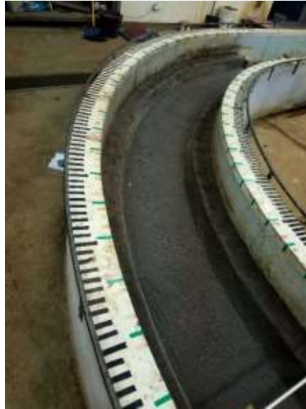
Gambar 64. Flume Model Sungai
