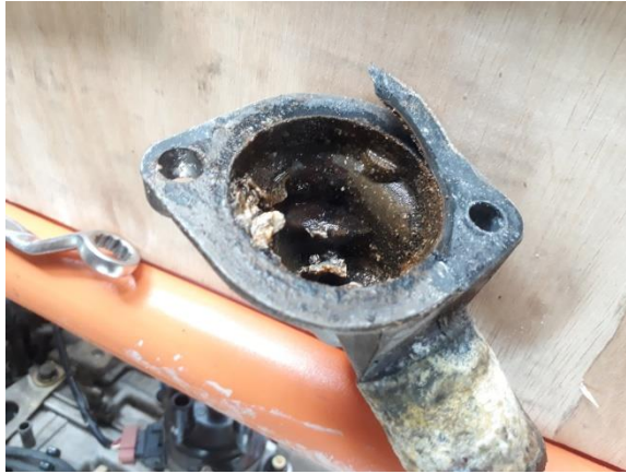
Gambar 10. Gasket TutupThermostat Robek
