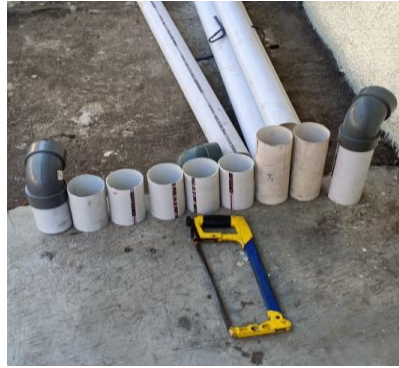
Gambar 7. Memotong Pipa Saluran Gas Buang
