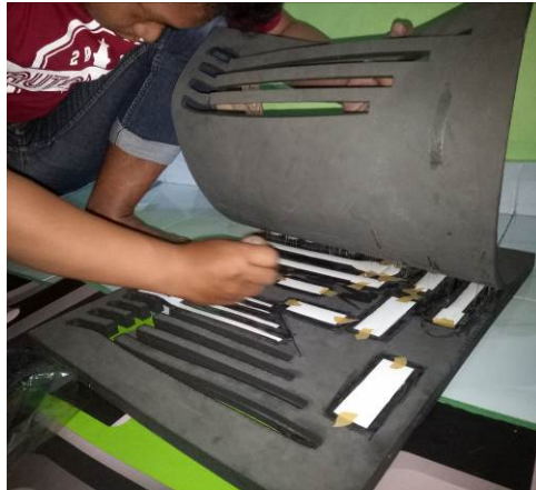
Gambar 12. Proses pengeleman busa hati
