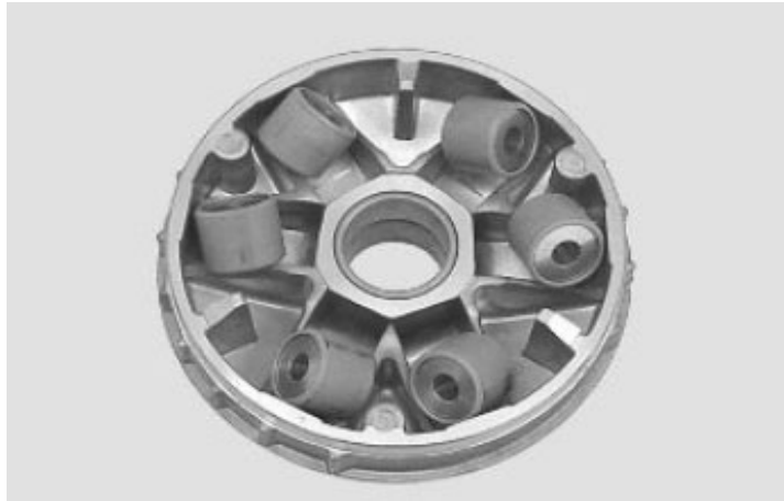
Gambar 5. Pulley bergerak / movable drive face (Sportworks, 2011)
