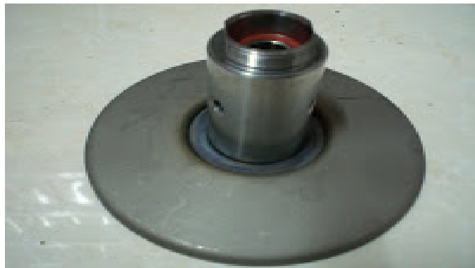
Gambar 11. Dinding dalam Pulley sekunder/ Secondary fixed Sheave ( Sportworks , 2011)
