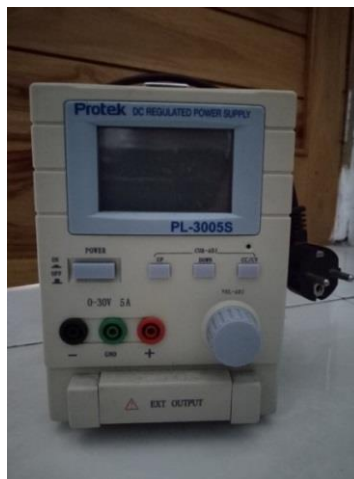
Gambar 16. DC power supply /catu daya DC
