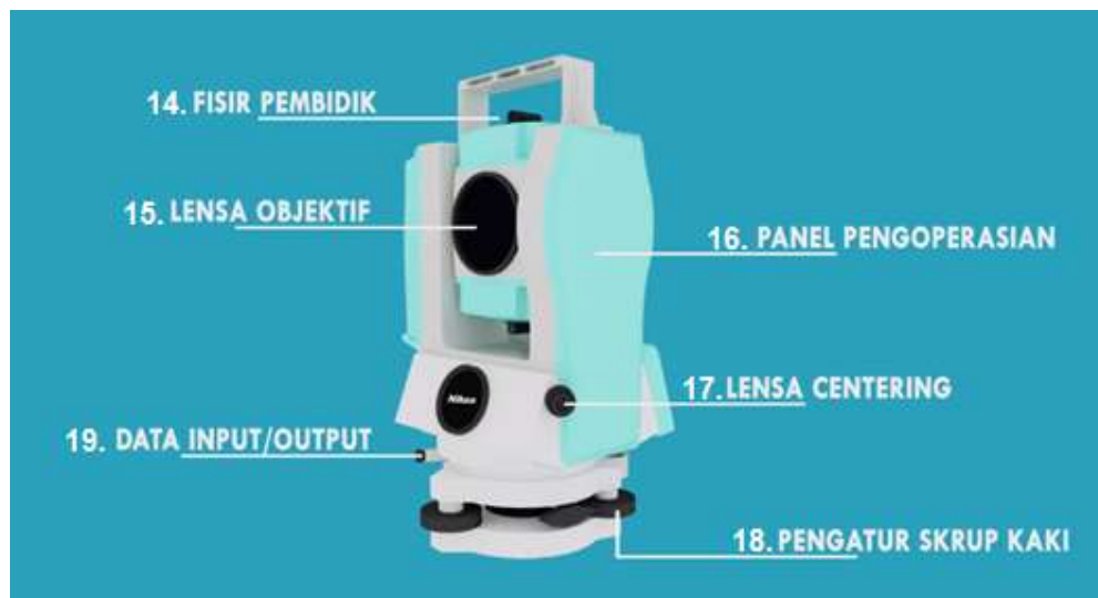
Gambar 3. Bagian-Bagian Total Station ( Trimble Navigation Limited Engineering and Construction Division: 2008 )
