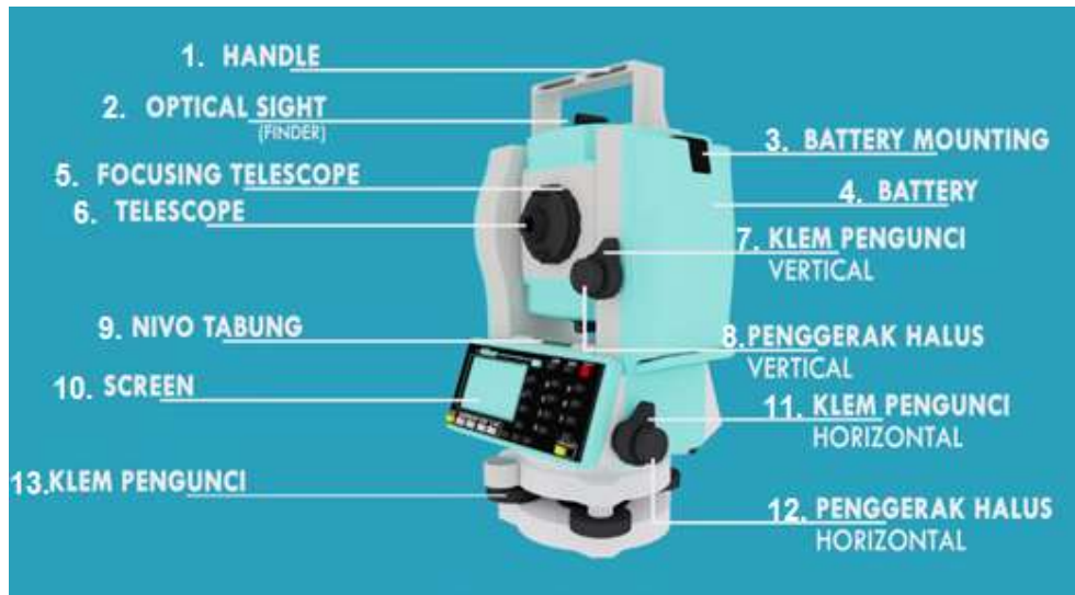
Gambar 2. Bagian-Bagian Total Station (Trimble Navigation Limited Engineering and Construction Division: 2008 )
