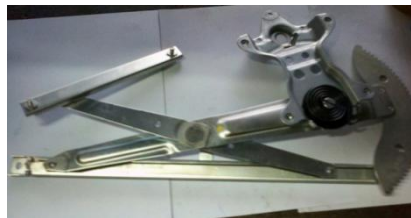
Gambar 10. Regulator Power Window Mekanis Sumber: tangomotor.com
