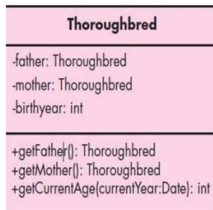
Gambar 5. Contoh class diagram (Pressman, 2012:988)
