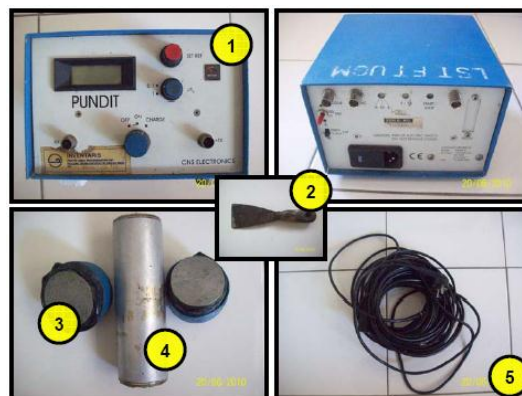
Gambar 22. Portable Ultrasonic Non-destructive Digital Indicating Tester (Sumber: Faqih, 2010)
