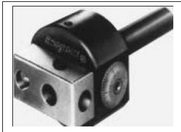
Gambar 13. Gambar Offset Boring Head (Widarto. 2008: 197)
