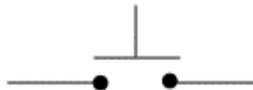
Gambar 12. Simbol Push-button PTM (Caang Go, 2011)
