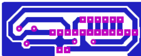
Gambar 31. Layout PCB LCD
