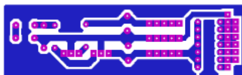
Gambar 25. Layout PCB regulator
