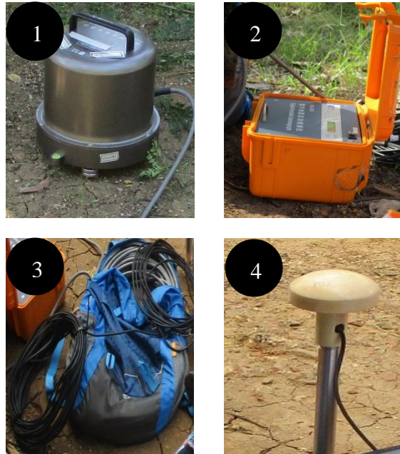
Gambar 10. Digital Portable Seismograph merk Taide tipe TDL-303S (1) Seismometer (2) Digitizer (3) Kabel penghubung (4) Antena GPS.
