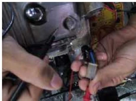
Gambar 63. Mengukur Tahanan Generator Pulsa
