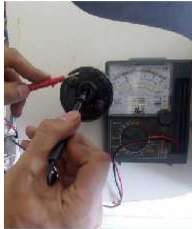
Gambar 61. Mengukur Tahanan Sekunder Coil
