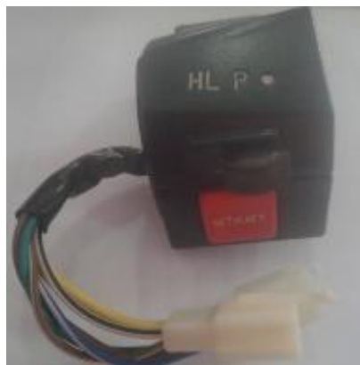
Gambar 09. Saklar Starter Sumber : ( https://www.google.co.id/search?biw=saklar+starter+astrea )
