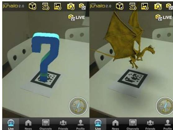
Gambar 2. Contoh marker based tracking
