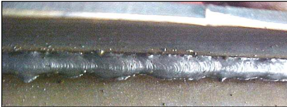
Gambar 2.10 contoh cacat incomplete fusion
