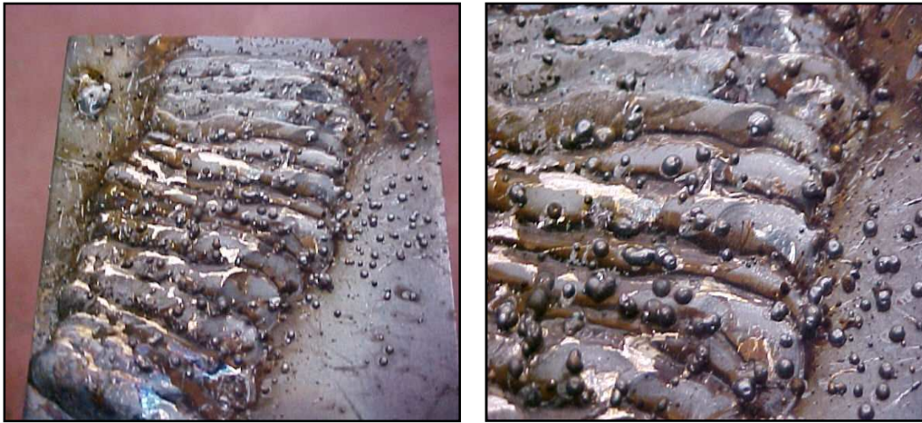
Gambar 2.6 cacat over spatter
