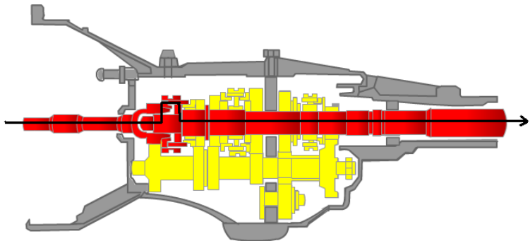
Input Shaft > Top gear > Hub Sleeve > Clutch hub > Main shaft
