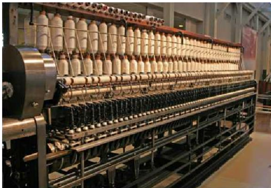
Gambar 2.4 Mesin Pinal (Spaining)
