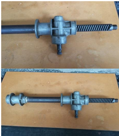
Media Roda gigi kemudi tipe Rack and Pinion
