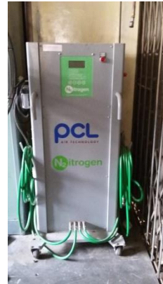
Nitrogen Generator Tyre
