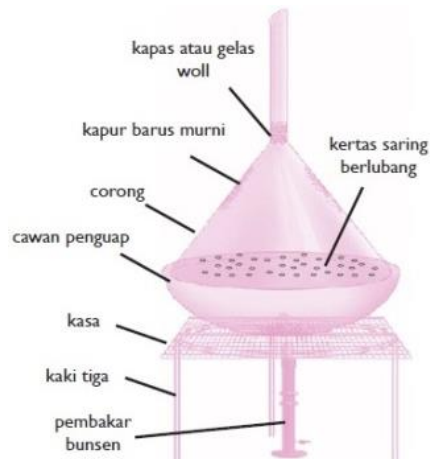
Gambar 8. Proses Sublimasi (Sumber gambar: https://image.slidesharecdn.com/ipasublimasikel-150304081515-conversion-gate01/95/ipa-sublimasi-kel-5-6-638.jpg?cb=1425478577 ) e. Sentrifugasi
