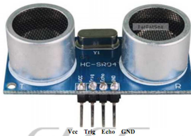
Gambar 7. Sensor Ultrasonic HC-SR04 Sumber: Datasheet HC-SR04
