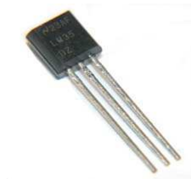
Gambar 4. Sensor Suhu LM35
