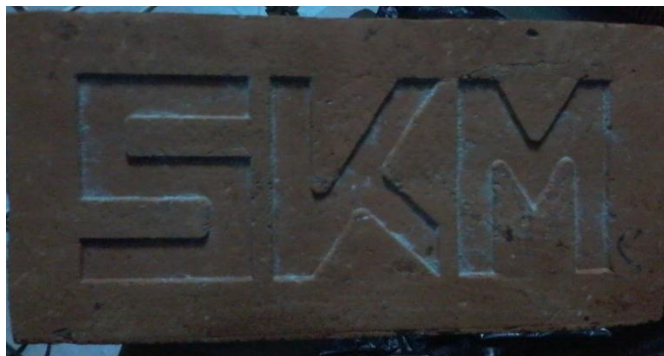
Gambar 3. Bata merah press/ekspos tipe SKM
