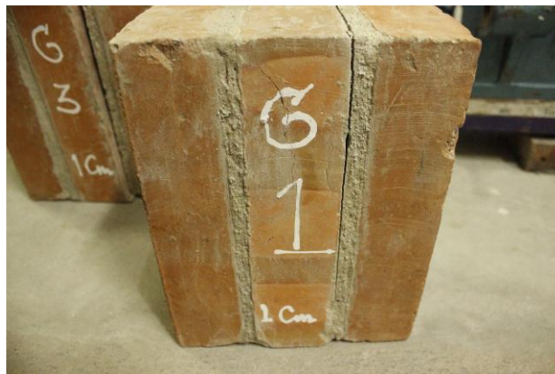
Gambar 58. Benda Uji 1GPB A 1PC:3Ps:3Pm
