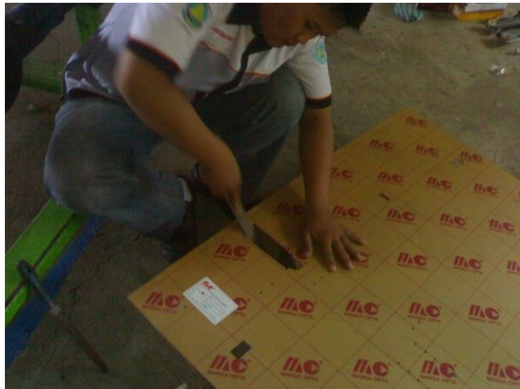
Gambar 26. Proses pengikiran acrylic
