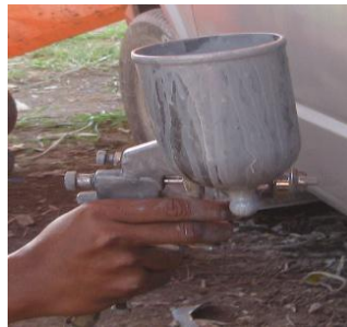
Gambar 14. cara memegang spray gun
