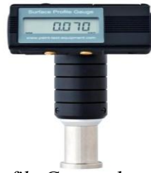
Gambar 16. Surface Profile Gauge alat ukur kerataan permukaan cat (Anonim, tth-b)
