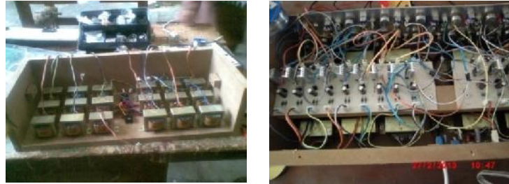
Gambar 43. Perakitan Power Supply .
