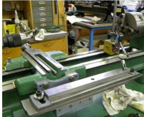
Gambar 36. Plain Taper Attachment
