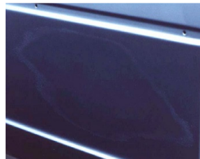
Gambar 48. Cacat tanda dempul (Sumber http://pc.dupont.com/dpc/en/US/html/visitor )
