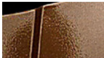
Gambar 44. Cacat kulit jeruk http://pc.dupont.com
