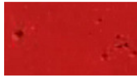
Gambar 47. Cacat pinholes http://pc.dupont.com
