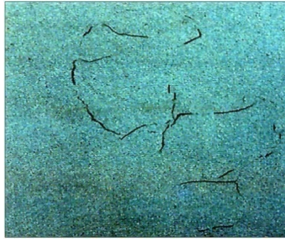
Gambar 49. Cacat goresan amplas (Sumber http://pc.dupont.com/dpc/en/US/html/visitor )
