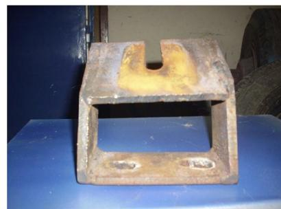
The purpose of the manufacture of engine mounting cradle that is used in the Toyota Corona with Toyota Kijang 3K engine is to assist students in designing engine mounting for vehicle modifications and restore the function of a Toyota Corona, so it can be used as a medium for the practice of engine tune up for the students of Automotive Engineering Study Program particularly in UNY.
