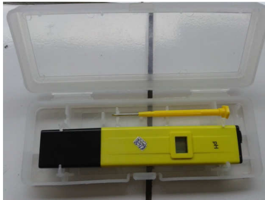
Gambar 7. pH meter Digital model pH-108 merk ATC
