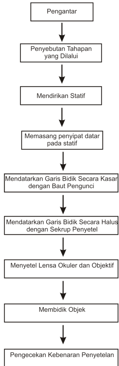
Gambar 9. Diagram Alir Media Audio Visual Setting Up Waterpass
